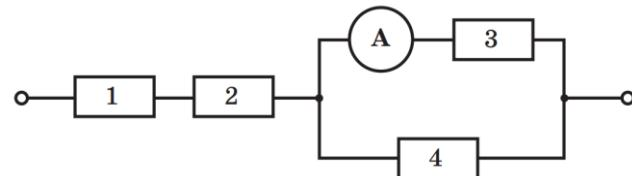
$$I_3 = 2 \text{ A} \quad U_3 = I_3 \cdot R_3 \quad [U_3] = A \cdot 0\Omega = A \cdot \frac{B}{A} = B$$
